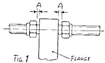
This procedure goes for the members B, C and D on both sides of the wheel. It is not necessary to correct the members simultaneously, but if the correction needed is great, say more than 1/8", repeat the procedure.
