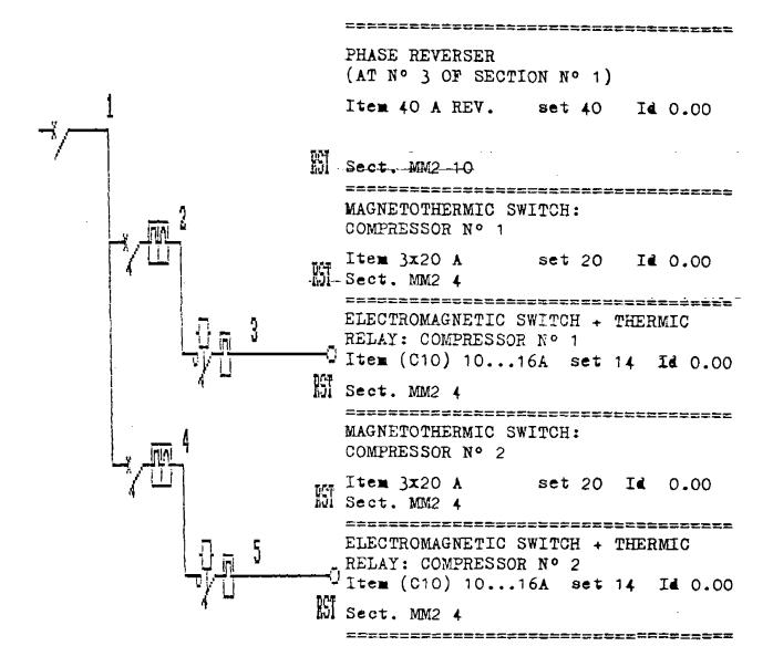
NOTICE: IN THE FOLLOWING SWITCHBOARD DIAGRAM (SECTION Nº 5) (COMPLETION OF SECTION Nº 1), THE HYDRAULIC PUMP SWITCH Nº 1 CORRESPONDS TO HYDRAULIC PUMP MAGNETOTHERMIC SWITCH INDICATE AT Nº 4 OF THE SWITCHBOARD DIAGRAM SECTION Nº 1.
