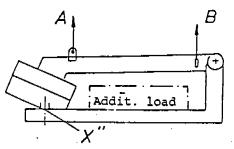
Lifting loads:  $A = 2 \times 9 \text{ tons}$   $B = 2 \times 6.3 \text{ tons}$ 30.5 tons
