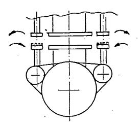
The two rotating parts of the gondola linkage are secured against each other by a locking frame.
